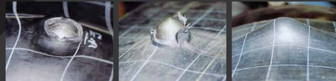
Nylon Fabric Belt (Retained Strength: 0%)
