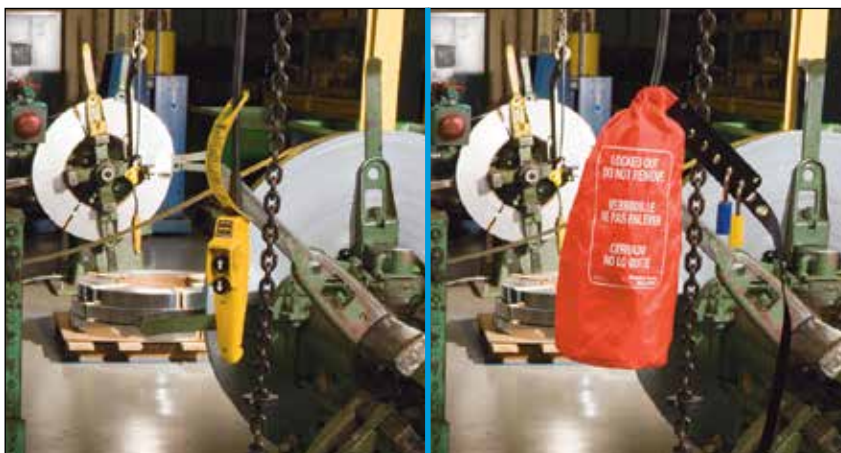
Hoist Control Cover
