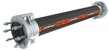
The hosing meets all the state-of-the-art equipment requirements for use at combination mining and beneficiation facilities, gold refining plants, and in other sectors. Hoses are connected together using aluminum couplings. The seal is maintained by a rubber-lined steel sealing ring.
