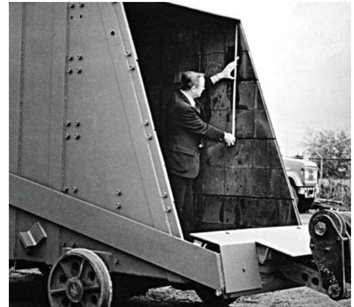
Don Wilding (the original inventor) in a Domite Lined Blast Furnace Skip, material handled Coke & Iron Ore. Photo c. 1970
