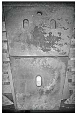
Jaw Crusher Cheek Plate
