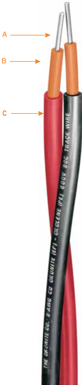
A Solid Uncoated Copper Conductors B Insulation - Okonite-Sizes #9 AWG and #8 AWG-5/64", #6 AWG-6/64" C Jacket-Okolene, Color Coded; 1-Black, 1-Red
