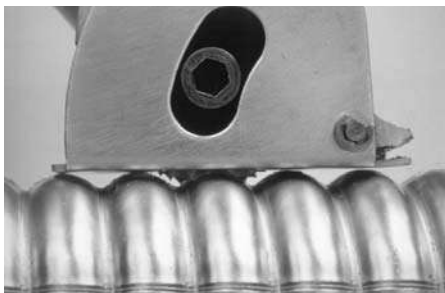
Set blade to remove 80 to 95% of the metal thickness in the valley.
